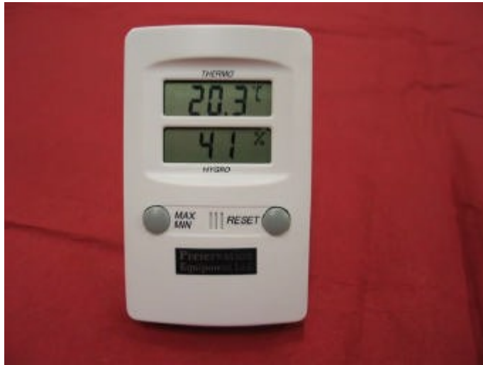
Device for monitoring temperature and humidity
